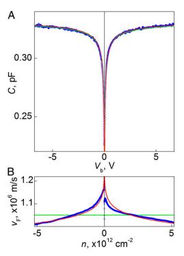
**Fig. 2.** Quantum capacitance of graphene. (*A*) Differential capacitance in zero *B*. Blue symbols are experimental data; green and red curves are the best fits with constant and renormalized  $v_{\rm F}$ , respectively. This particular device has  $d\sim27$  nm and  $S\sim250~\mu{\rm m}^2$ . (*B*) Same data replotted in terms of  $v_{\rm F}$  and carrier concentration n; color coding as in A.
