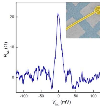
Figure S8. Valley-based transistor. Nonlocal resistance as a function of top gate voltage  $V_{top}$ . The inset shows an electron micrograph in false color of the measured superlattice device. G/hBN is in light blue, and the top gate is in gold.  $L \approx 4 \mu\text{m}$ ;  $w \approx 1 \mu\text{m}$ ;  $T = 20 \text{ K}$ . The thickness of the top hBN dielectric is  $\approx 15 \text{ nm}$ . The back gate voltage is close to zero but is slightly tuned to reach the main NP.
