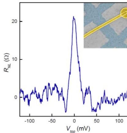
Figure S8. Valley-based transistor. Nonlocal resistance as a function of top gate voltage  $V_{top}$ . The inset shows an electron micrograph in false color of the measured superlattice device. G/hBN is in light blue, and the top gate is in gold.  $L \approx 4 \mu\text{m}$ ;  $w \approx 1 \mu\text{m}$ ;  $T = 20$  K. The thickness of the top hBN dielectric is  $\approx 15$  nm. The back gate voltage is close to zero but is slightly tuned to reach the main NP.
