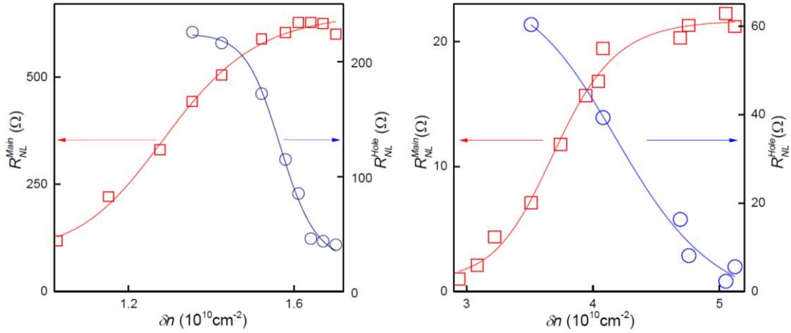
Figure S5. Nonlocal transport in graphene superlattices as a function of charge inhomogeneity.  $\delta n$  is determined from broadening of the resistance peak at the main NP and quantified by fitting it with the dependence  $\rho_{xx}(n) \propto 1/(n^2 + \delta n^2)^{1/2}$ . Left and right panels are for G/hBN devices with  $L \approx 3.5 \mu\text{m}$  (encapsulated) and  $5 \mu\text{m}$  (non-encapsulated), respectively.
