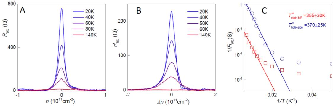
**Figure S3.** Temperature dependence of nonlocal resistance  $R_{NL}$  at the main (**A**) and hole-side (**B**) NPs. Encapsulated G/hBN device;  $w \approx 1 \mu\text{m}$  and  $L \approx 3.5 \mu\text{m}$ . The carrier density  $\Delta n$  in (**B**) is counted from the position of the secondary NP. (**C**) Detailed  $T$  dependences for the peaks in (**A**) and (**B**).
