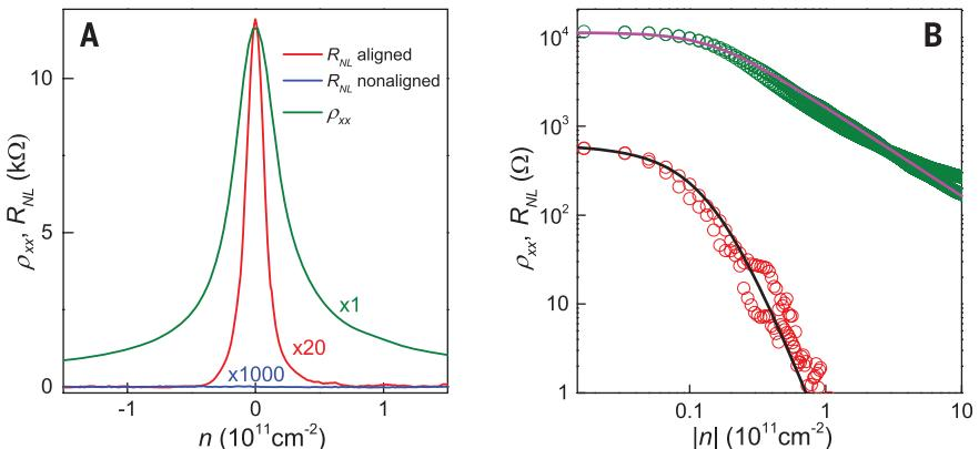
**Fig. 2. Density and distance dependences for nonlocal valley currents.** (A)
