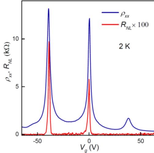
Figure S1. Resistivity  $\rho_{xx}$  and nonlocal resistance  $R_{NL}$  in zero magnetic field. The data are for non-encapsulated superlattice device with  $w \approx 1 \mu\text{m}$ .  $R_{NL}$  was measured at separation  $L \approx 5 \mu\text{m}$  (see the device geometry in Fig. 1 of the main text).
